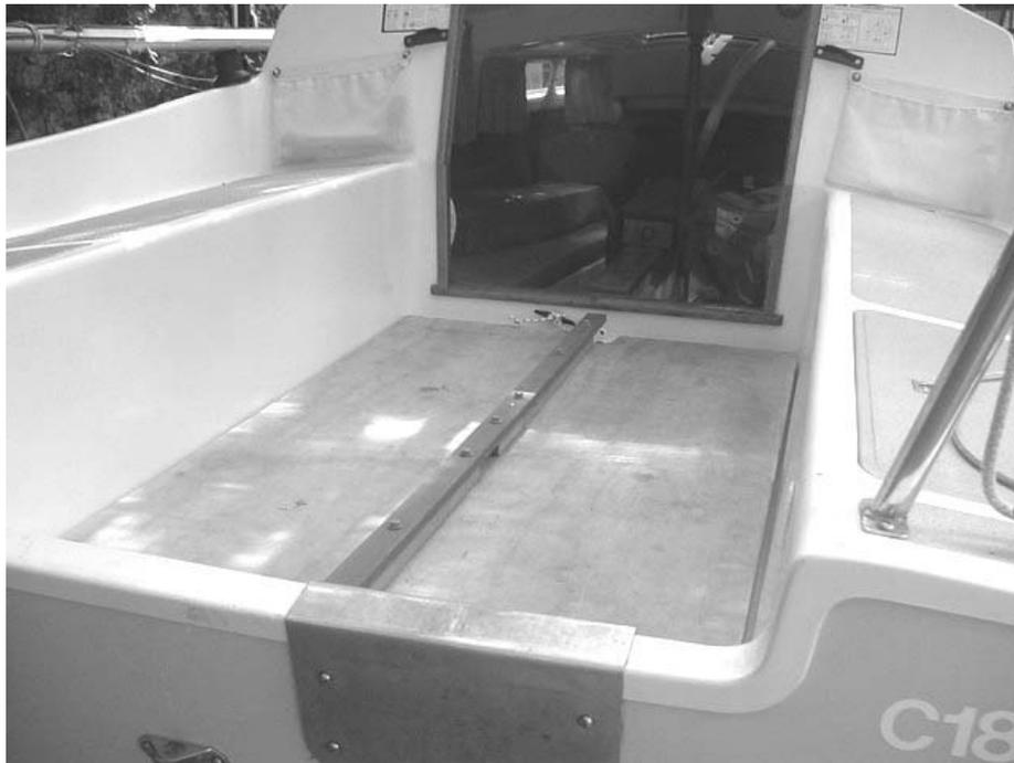
Then flip the sheet of ply over, so the bracing strip is on the bottom. Those gaps "strategically placed" in the lengths of cypress allow you to feed the support strips through, so they won't slide around (though this shouldn't be a problem). Note that this process is a bit awkward. If you didn't want the bracing strip, you would avoid having to flip the ply sheet.
